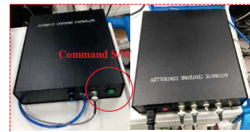
Fig. 4 Manufactured control box for the impact actuator
