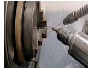
Fig.3. High precision grinding and polishing Table 3. The parameters of high precision grinding and polishing
