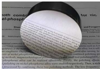
Fig. 4 Nickel-phosphorus surface after combined polishing process
