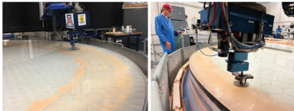
Fig. 3 GMT Segment 3 being polished with a 40 cm pitch lap at left and a 10 cm lap at right. Both laps are driven by the same orbital polisher [25].
