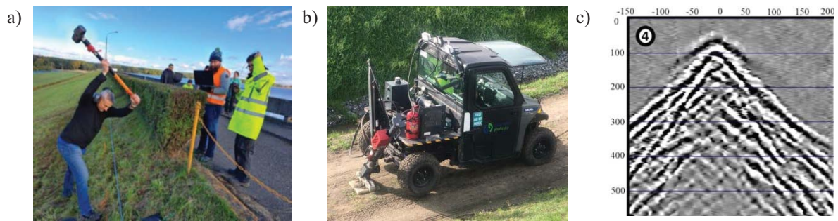
Fig. 6. a) Manual vibration source; b) seismic vibrator truck; c) example DAS signal both in length and time domain.
