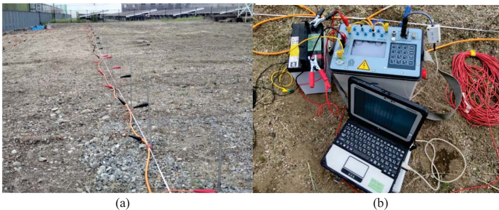
Fig. 5. Electric resistance measurement; (a) Setup of electrodes; (b) Resistivity meter.
