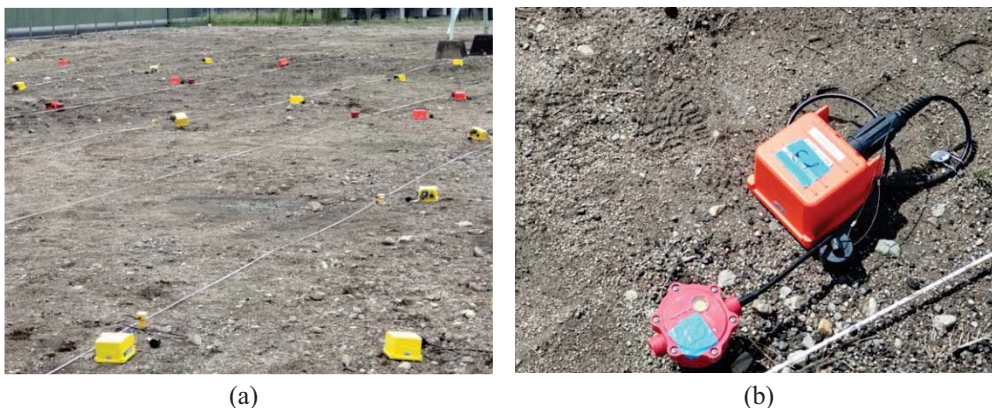
Fig. 3. Ambient noise measurement; (a) Layout of geophones; (b) Three component geophones.
