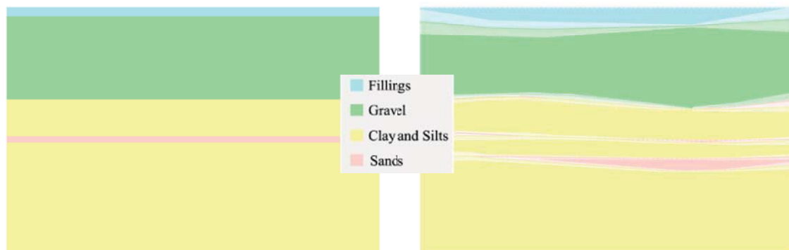
Figure 2. Comparison of two approaches to subsoil modelling for the Munich Case Study with: (a) a deterministic 2D subsoil model as used in the original analysis, which presents fixed soil stratification, and (b) a probabilistic subsoil model that highlights uncertainty in soil stratification with the 95th percentile layer boundaries around the expected soil interfaces.
