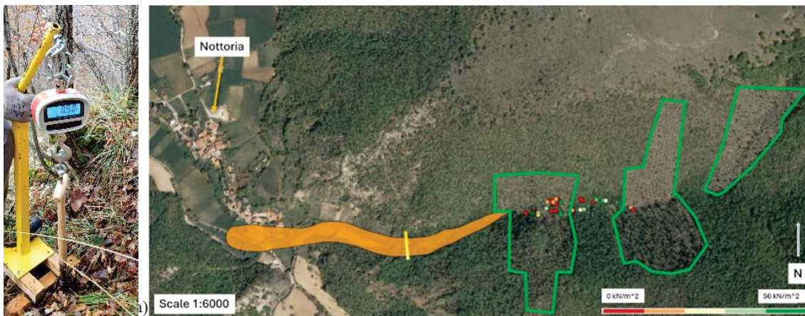
Figure 3. a) corkscrew equipment and b) investigated area of debris flow (marked by the orange polygon): the symbols refer to the cork-measurements (in kPa) inside and outside vegetation cutting areas (marked by the green polygons). The yellow line is the trace of a bridge built as a risk mitigation work.
