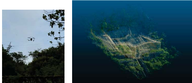
Fig. 1.(a) Data collection with UAV for 3D reconstruction and (b) reconstructed point cloud model of a rigid barrier.
