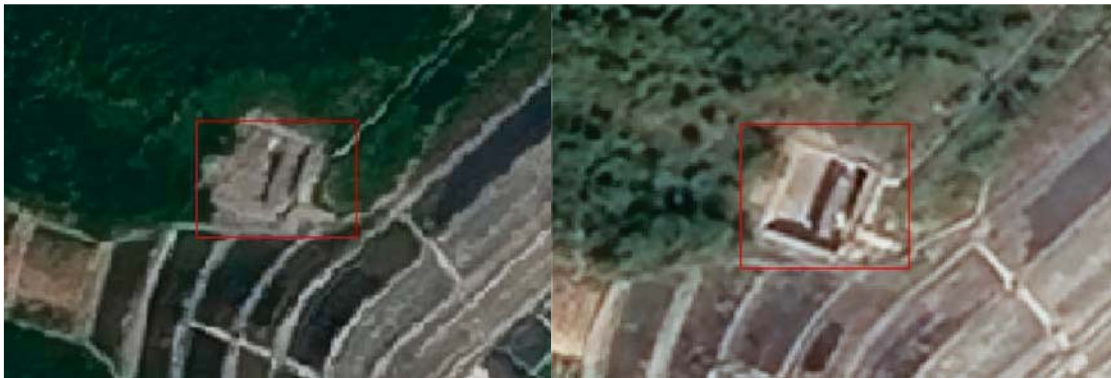
Fig. 3. Near-real-time monitoring of a typical rigid barrier (a) before the rainstorm and (b) after the rainstorm.
