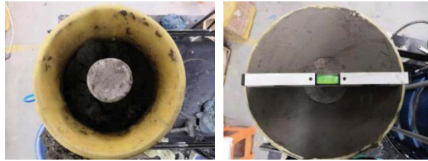
Figure 4. Specimen preparation of GCTS large-scale triaxial test: (a) sample preparation; (b) flatness calibration of sample top surface
