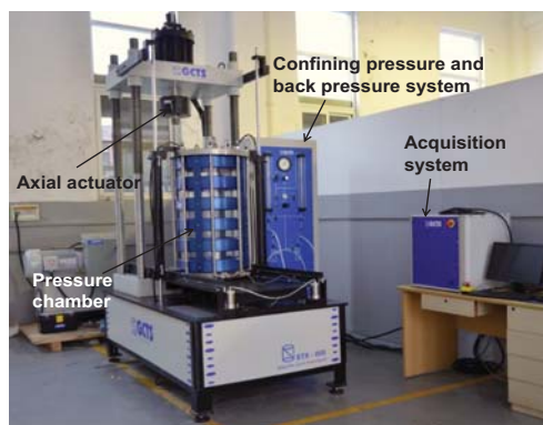
Figure 1. GCTS large scale triaxial apparatus
