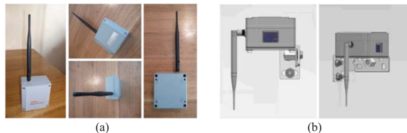
Figure 1. Data acquisition nodes object picture (a) tilt sensor; (b) laser ranging sensor
