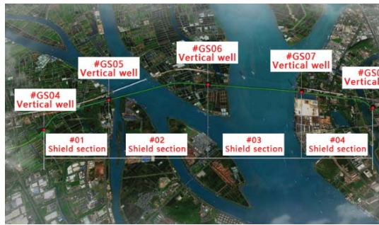
Figure 9. Tunnel roadmap of B3 section.
