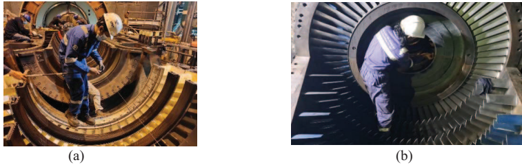
Fig. 3. casing alignment data collection process (a) Top off with piano wire (b) Top On with laser alignment tool.
