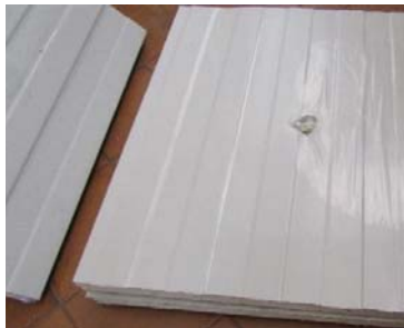
Figure 9: ribs present on external steel sheets of panels.
