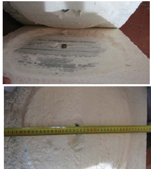
Figure 5: de-bonding of polyurethane after the impact.
