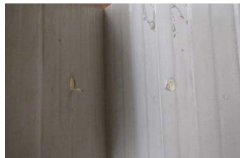
Figure 6: double layer panels uncoupled after impact, unperforated second panel (right)
