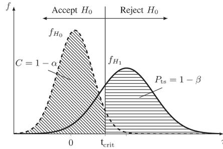
Fig. 1. Relationships of  $f_{H_0}$  &  $f_{H_1}$  and the resulting integrals of  $C$  and  $P_{ts}$  (Grundler 2022)
