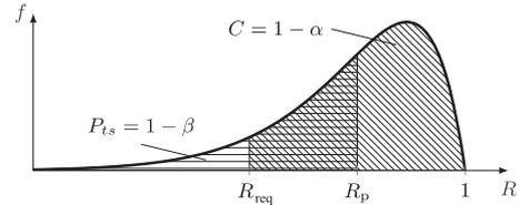
Fig. 2. Beta distribution of the SR test and the corresponding integrals for  $C$  and  $P_{ts}$  (Grundler 2022)
