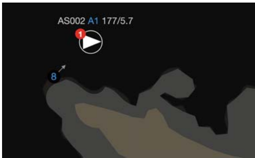
Fig. 4. High visual priority on the alarm, mid-level is dynamic data. Wind is indicated with arrow, and place of measurement. Bottom visual level is the static environment with black sea, dark grey is less than 10 m depth, land has a faded beige color.
