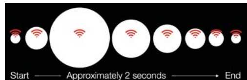
Fig. 7. Dynamic alarm-spot to attracting attention, Here placed on top of a red Wi-Fi symbol for a connectivity problem.
