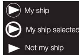
Fig. 1. The ship points (metaphor) in its sailing direction. Distinguishing between my own ship, a selected ship “click” and other ships.
