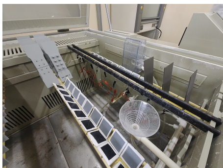
Fig. 2. Accelerated salt spray aging test equipment for silicone rubber.
