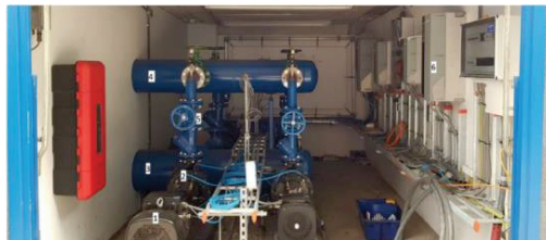
Fig. 7. Experimental set-up of e-motor driven centrifugal pumps equipped with multiple sensors.
