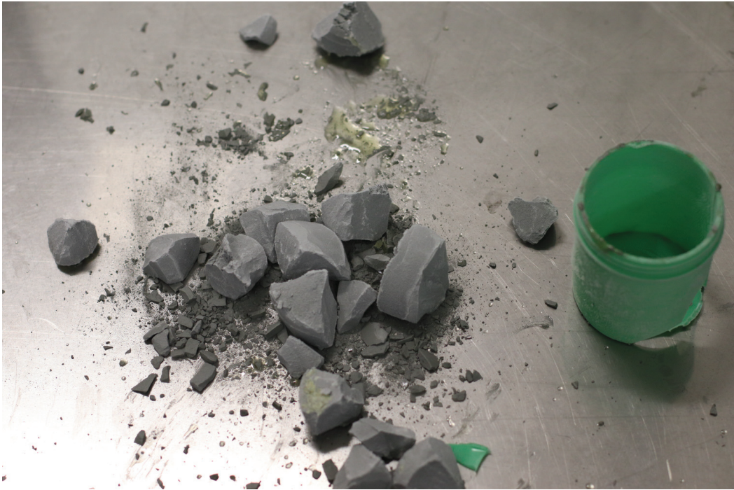
Fig. 3. Separation of solder paste from the solder paste container with liquid nitrogen: Frozen solder paste separated from the solder paste container by mechanical treatment
