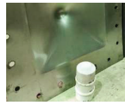
Figure 4: Example of a passed impact test, material sample and projectile, source: JMTBA, Japan
