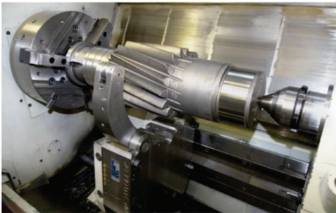
Fig. 1. Chuck and quill with 600 kg workpiece, source: A.Monforts, Mönchengladbach
