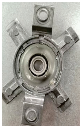
Fig 9. Debris from washer wear out after component failure
