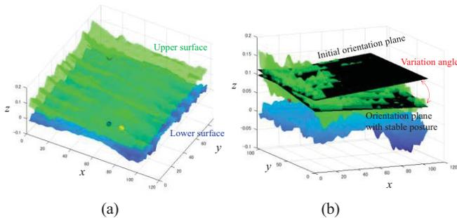
Fig. 1 Contact simulation between two surfaces: (a) Example of two surfaces and contact points in a simulation, (b) Example of variation angle of the upper surface from its initial position.
