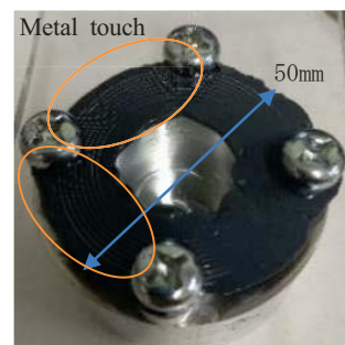
Fig. 1 Example of the flange after metal touch by the seal material.
