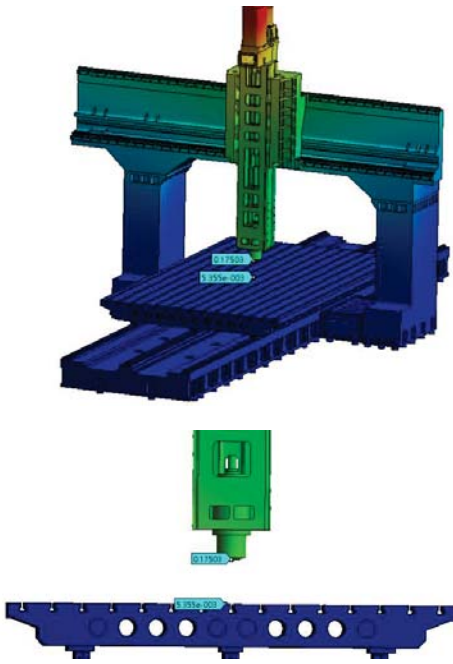
Fig.4 Static analysis - X axial cutting force 5000N
