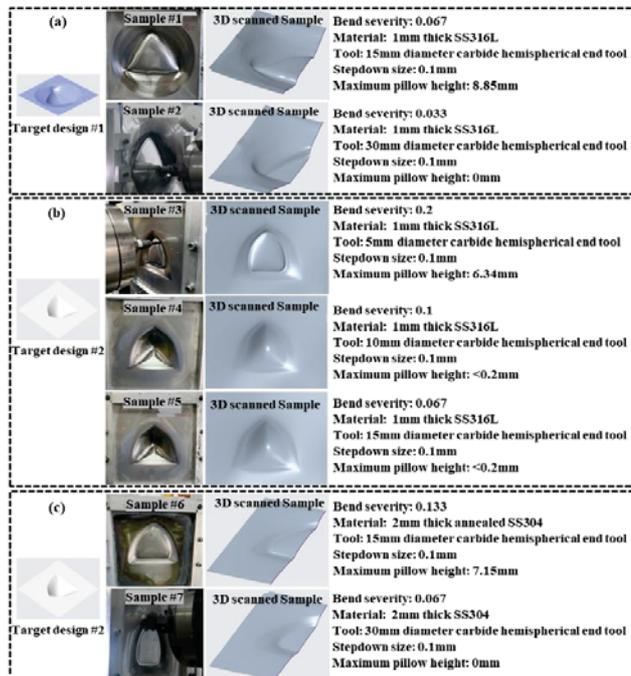
Fig. 6 Effect of bend severity on pillow formation for different samples: (a) Samples #1 and #2; (b) Samples #3 to #5; and (c) Samples #6 and #7.
