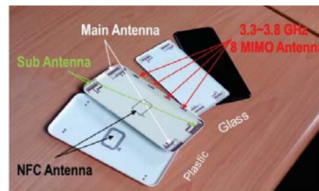
Fig. 2 A multi-band 4 MIMO antenna and a NFC antenna on plastic/glass back cover of mobile phone.
