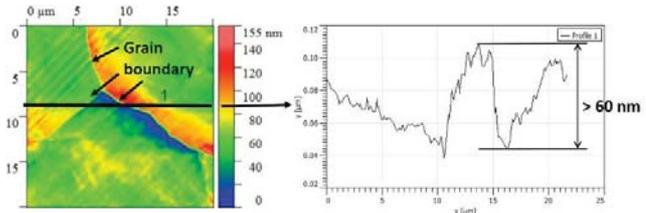
Fig. 3 Grain boundary steps of polycrystalline tin after SPDT
