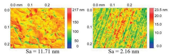
Fig. 4 Surface topography of polycrystalline tin after SPDT. (a) Unmodified surface; (b) Laser-based modified surface.
