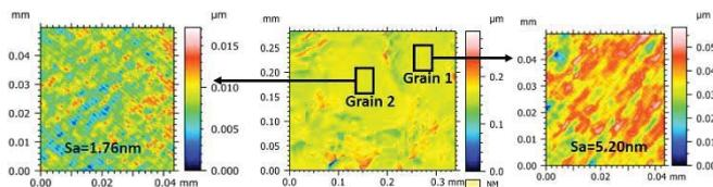
Fig. 2 Surface topography of polycrystalline tin after SPDT
