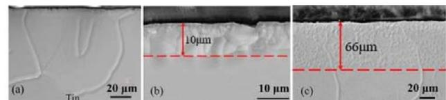
Fig. 5 SEM images of cross-sectional samples. (a) Unmodified subsurface; (b) Modified subsurface with laser beam with low power density ( $2.1 \times 10^4 \text{ W/mm}^2$ ); (c) Modified subsurface with laser beam with high power density ( $3.9 \times 10^4 \text{ W/mm}^2$ ).
