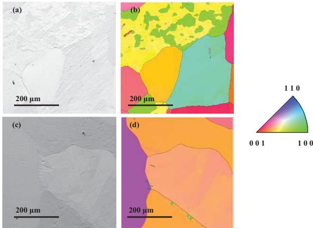
Fig. 8. Characterization of polycrystalline tin surface. (a) SEM image of the  $500 \times 500 \mu\text{m}$  area in unmodified sample; (b) EBSD IPF map of the same surface in (a); (c) SEM image of the  $500 \times 500 \mu\text{m}$  area in modified sample; (d) EBSD IPF map of the same surface in (c).
