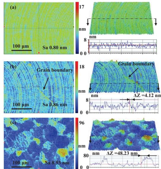
Fig. 7. Surface roughness in Sa under orthogonal optimal parameters. (a) After plasma treatment and in one of grain; (b) After plasma treatment and at the junction of two grains; (c) Without plasma treatment.
