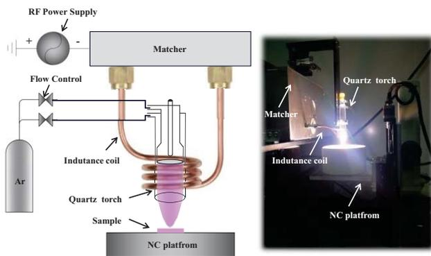
Fig. 6. Schematic diagram and photograph of ICP setup.
