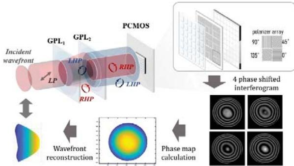
Fig. 1 Dynamic wavefront sensor based on a geometric phase lens pair; GPL, geometric phase lens; PCMOS, polarization pixelated camera; LP, linear polarization; LHP, left-handed circular polarized; RHP, right-handed circular polarized. The inset describes an inner polarizer array of the PCMOS.
