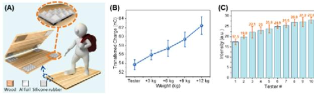
Fig. 3 (A) Configuration of the weight sensing mat containing four silicone rubber-pyramid units. (B) Relationship between the obtained transferred charge and the individual (50 kg) holding varying weights of objects from 3 kg to 12 kg. (C) The measured result of 10 users with different weights when connecting the sensing mat to MCU.
