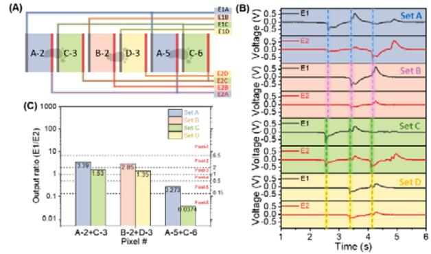
Fig. 2 (A) Schematic illustration of interval arrangement of four sets of mats for arbitrary walking monitoring. (B) Triboelectric output of the four sets (8 electrodes). (C) Corresponding output ratios when a user walks along the mat array with a manner of one step two pixels.
