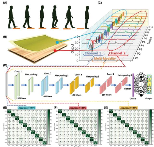
Fig. 4 (A) Schematic illustration of a normal walking step including stepping on the entry mat, standing still and stepping off. (B) Configuration of the entry mat. (C) Corresponding outputs from the two channels during a normal walking step for 10 users. (D) Structural illustration of the convolutional neural network (CNN). (E)-(G) Confusion maps obtained using (E) channel 1 only, (F) channel 2 only, (G) multi-modality analysis of channel 1 and channel 2.
