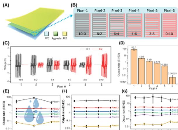
Fig. 1 (A) Structure of a single mat pixel. (B) Diagrams of six IDE patterns with different finger width ratios in one mat set: (C) Triboelectric outputs from two output electrodes of 6 individual pixels. (D) Corresponding output ratios (E1/E2) extracted from C. (E) Output ratios under varying humidity. (F) Output ratios under varying contact weight. (G) Output ratios from different stepping positions (middle, upper left, upper right, bottom right, bottom left).
