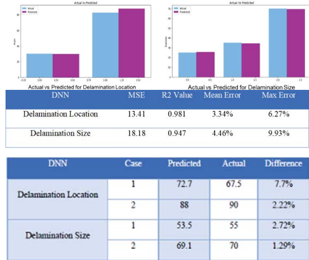
Fig.8 ANN prediction performance on delamination conditions
