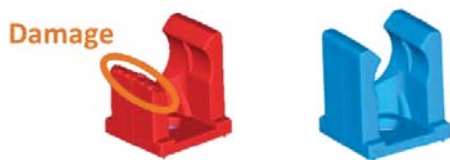
Fig. 1 X-ray CT scan data (left) and CAD data (right) with different shapes
