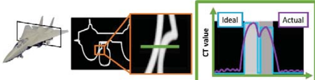
Fig. 3 Blurred boundary (left: scanned object, center: CT volume and enlarged image, right: the change in CT value)
