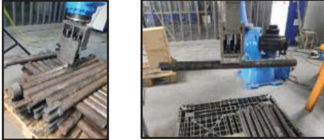
(a) Adsorbing the camshaft (b) Picking up the camshaft
