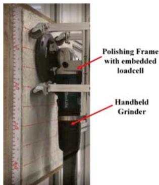
Fig. 7 Line grids on concrete specimen to aid in analyzing linear grinding speed
