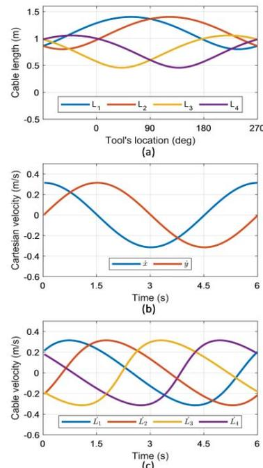
Fig. 3 (a) Required cable lengths to perform a circular path tracing ( $r=0.3m$ ), (b) EE cartesian velocity, (c) EE joint velocity.
