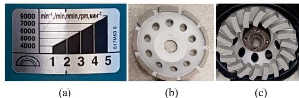
Fig. 6 Grinder's variable speed controller and 5 inch Low-Vibration Diamond Cup Wheel (b) Single Row and (c) Turbo
