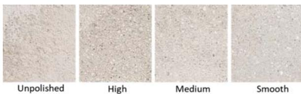
Fig. 8 Visual indication of surface roughness, before (unpolished) and after (high, medium, smooth) polishing
