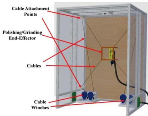
Fig. 1 Conceptual design of the cable-driven manipulation system for wall polishing and grinding
