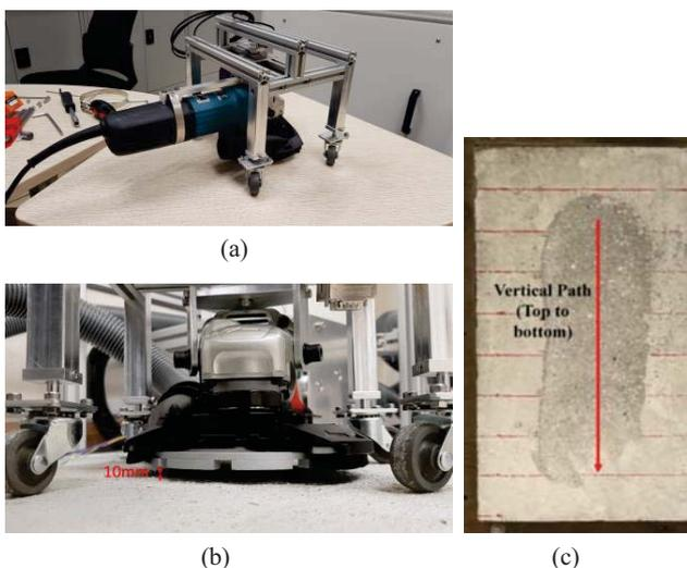
Fig. 5 (a) Polishing frame (b) There is a 10mm distance between the grinding media and the wall surface when force is not applied (c) Grinding trial path on concrete specimen
