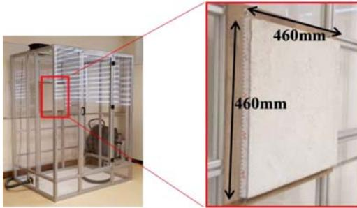
Fig. 4 Experimental test setup with concrete wall specimen
