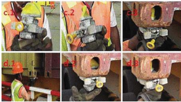
Fig 1. Removing and fixing the twist-lock from and to the corner cast of the container is an example of a task requiring coordinated dual arm manipulation navigating through tight spaces.
