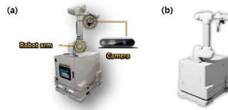
Fig. 3 Realization of the actual camera-mounted robot system into DT; (a) real robot (Doosan M1013+Realsense D415), (b) DT robot
