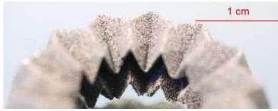
Figure 3. Cooling channel in NdFeB part fabricated using AM [3]
