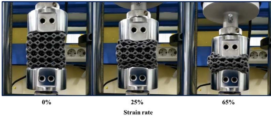
Fig. 3. Compressive deformation images of compression test with specimen No. 25
