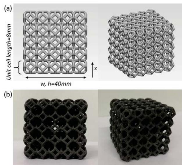
Fig. 2 Kelvin lattice cube-shaped of (a) CAD, (b) as-printed specimen
