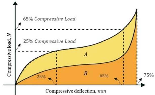
Fig. 1. Load-deflection curve of TPU Kelvin structure
