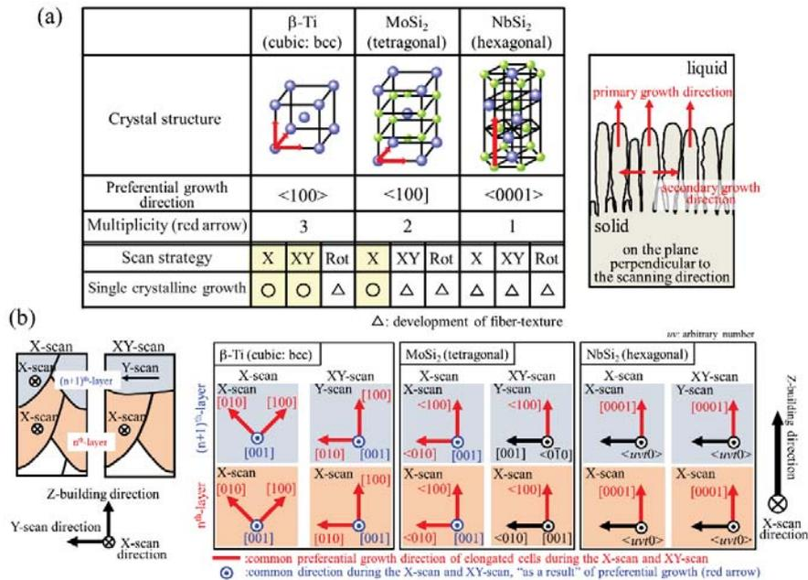
Fig. 1 (a) Relationship among crystal structure, preferential growth direction of elongated cell, and texture developed in L-PBF.
