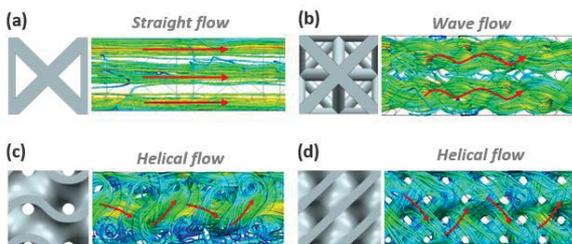
Fig. 5 Comparison of streamlines at  $Re = 32,500$  and heat rate = 70 W (a) FBCCz. (b) Octet-truss. (c) Gyroid sheet. (d) Diamond sheet.
