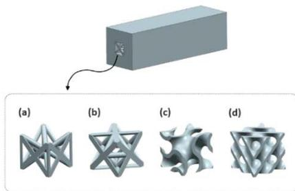
Fig. 1. Unit cells of cooling channel (a) FBCCz. (b) Octet-truss. (c) Gyroid sheet. (d) Diamond sheet.
