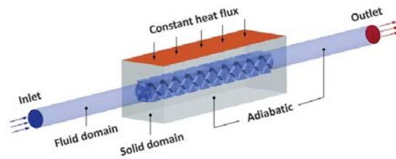
Fig. 3 Schematic of the CFD domain and boundary conditions
