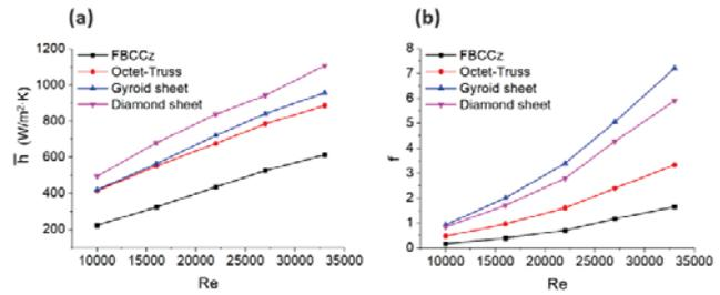
Fig. 6 Simulation results of (a) the overall heat transfer coefficient. (b) friction factor at different  $Re$ . and heat flux = 70 W.
