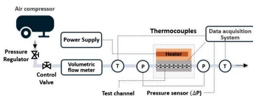
Fig. 2 Schematic of experimental set-up for metamaterial channels.
