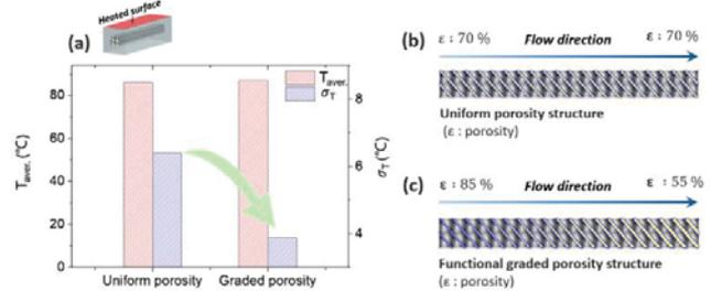
Fig. 7 Simulation results of (a) the heated surface temperature at  $Re = 32,500$  and heat rate = 70 W (Diamond  $\epsilon = 70\%$  vs Diamond  $\epsilon = 85\sim 55\%$ , Based on the same volume fraction). (b) Uniform porosity structure. (c) Functional graded porosity structure.
