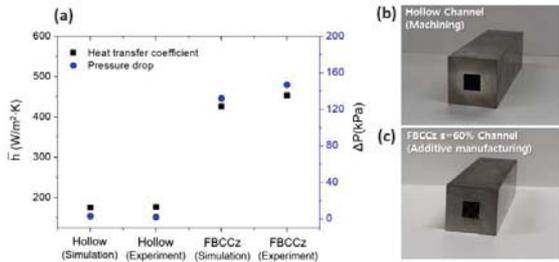
Fig. 4 Validation of (a) predicted heat transfer coefficient and pressure drop at  $Re = 32,500$  and heat rate = 30 W (Hollow vs FBCCz  $\epsilon = 60\%$ ).
