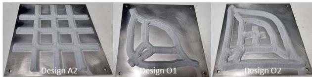
Figure 3 CSAM-built Al6061 stiffeners on Al6061-T6 panel
