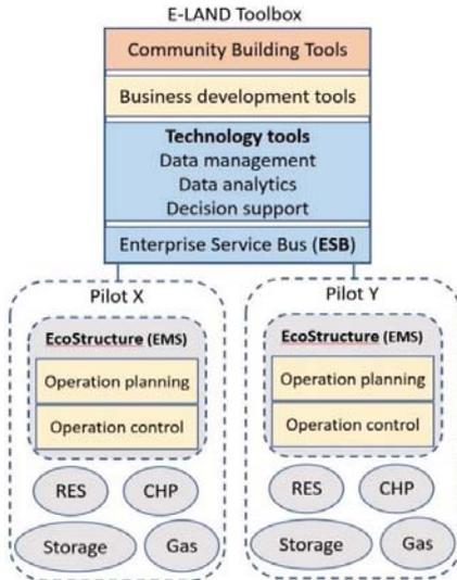
Fig. 1. E-LAND Toolbox high level architecture (Jørgensen et al.).
