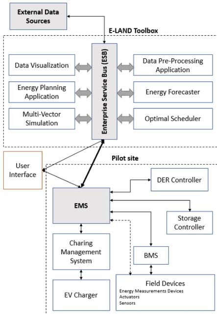
Fig. 2. Components of the E-LAND toolbox and the Pilot sites (Jørgensen et al.).
