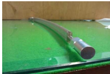
Fig. 1. Shape of pyro expanding tube.
