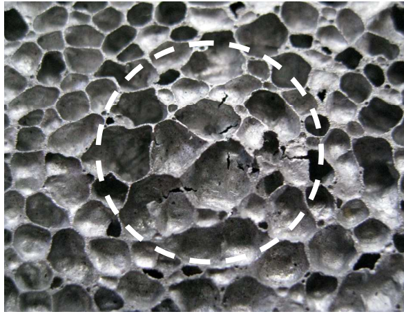
Fig. 7. Photograph of the back region of the sample tested with simple support boundary condition and FEP indentation with depth 6 mm.
