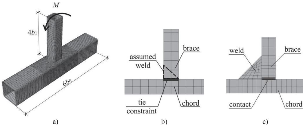
Figure 2. FE model: a) meshing; b) butt welds modelling, c) fillet welds modelling.
