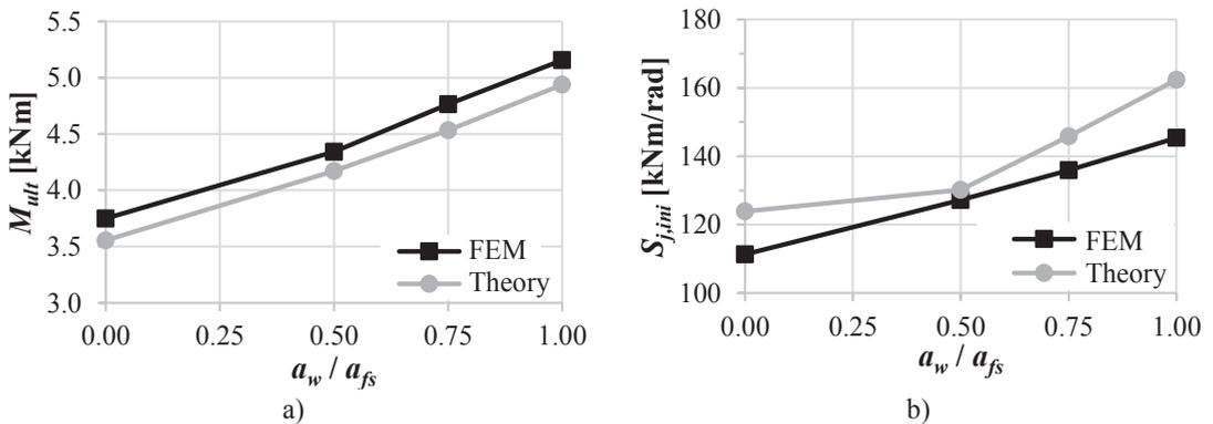
Figure 5. Determination of  $k_{fw}$  for joint 150x5-80: a) resistance ( $k_{fw} = 0.9$ ), b) initial stiffness ( $k_{fw} = 0.4$ ).  $a_w/a_{fs} = 0$  corresponds to a butt-welded joint.
