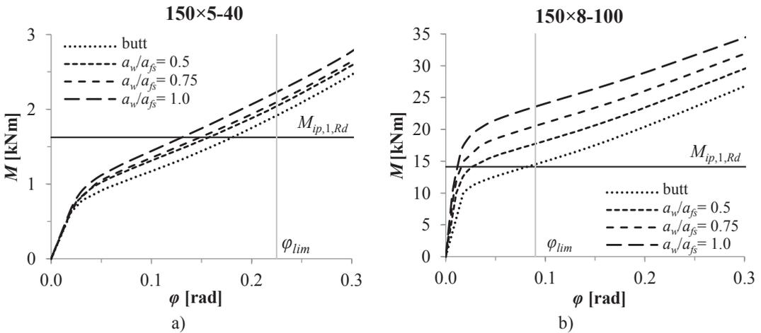
Figure 4. Load-displacement curves of T joints: a) 150×5-40-355 and b) 150x8-100-355.
