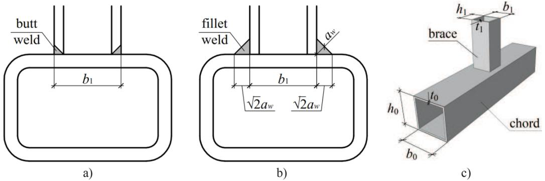
Figure 1. a) Idealized butt-welded joint; b) idealized fillet-welded joint; c) notations of RHS T joint.
