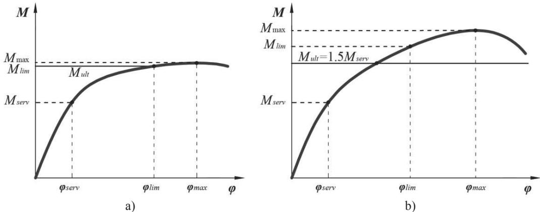
Figure 3. Resistance of RHS T joint: a)  $M_{lim}/M_{serv} \leq 1.5$ ; b)  $M_{lim}/M_{serv} > 1.5$ .
