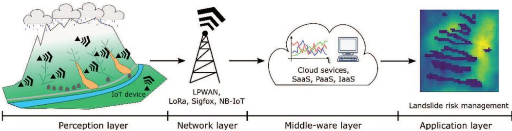
Figure 1. IoT architecture for a shallow landslide monitoring system.
