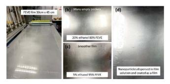
Fig. 4 Films coated using the roll-to-roll film coater (a) FEVE film (b) 20% ethanol mixed into 80% FEVE (c) 5% ethanol mixed into 95% FEVE (d) Nanoparticles infused film
