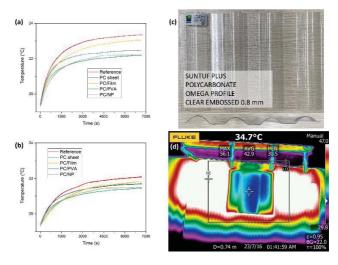
Fig. 5 Temperature measured by sensors in the modular acrylic enclosure simulating a greenhouse at a position (a) close to the LED lamp (b) 30 cm away from the LED lamp (c) actual photo of a PC sheet (d) IR image of the PC sheet after 1h of heating
