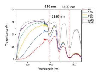
Fig. 2 UV-Vis spectrum of the NaYF<sub>4</sub>:Yb,Er UCNP dissolved in ethanol at varying concentrations and the FEVE resin
