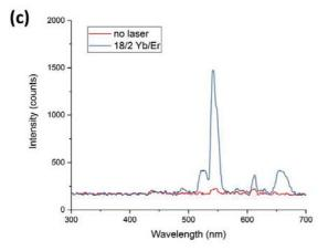
Fig. 3 (a) NaYF<sub>4</sub>:Yb,Er nanoparticles in ethanol before the 980 nm laser is switched on (b) Green visible light emission observed under 980 nm excitation (c) Fluorescence spectrum of the emitted light under 980 nm excitation
