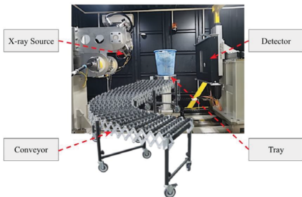
Fig. 2 Hardware schematic of X-ray scanning module.
