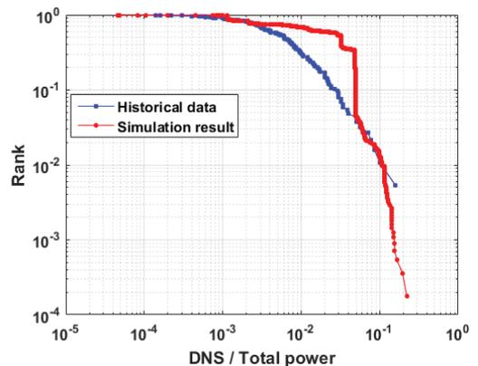
Fig. 3. Cumulative distribution of the DNS obtained with the cascading failure model for default  $\alpha$ .
