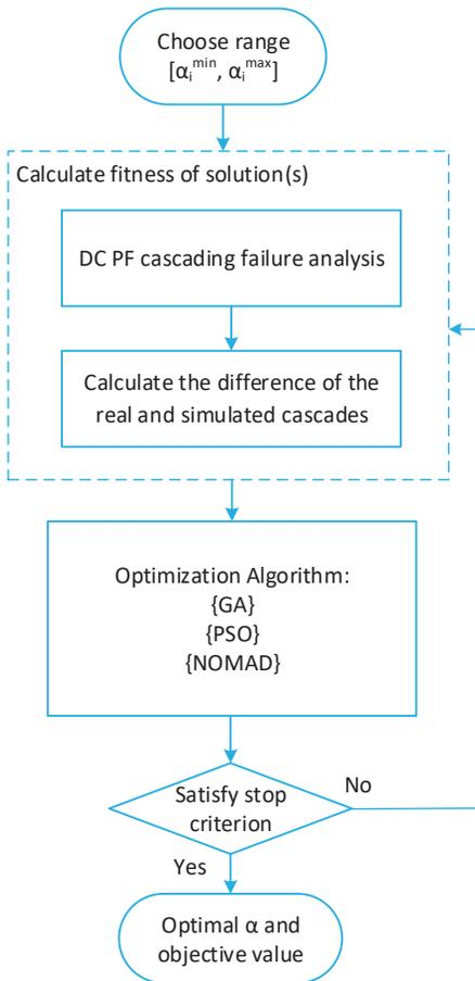
Fig. 2. Algorithm for the GA based calibration approach
