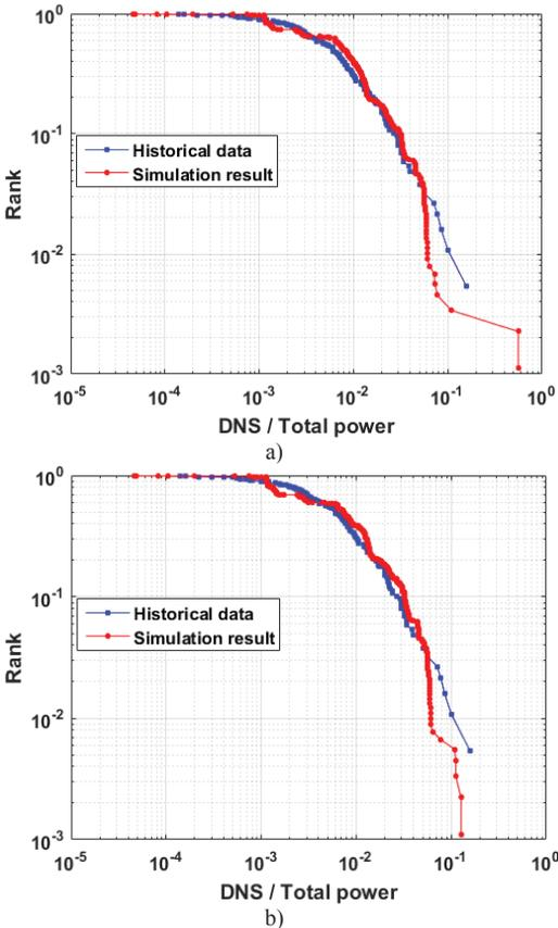
Fig. 4. Cumulative distribution of the DNS obtained with GA with: a) Minkowski distance; b) Kullback-Leibler divergence objective functions.
