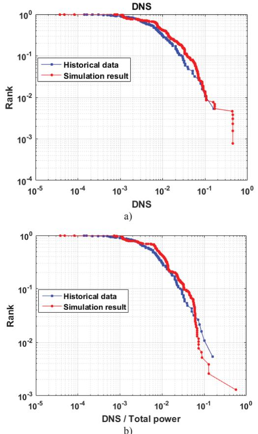
Fig. 5. Cumulative distribution of the DNS obtained with PSO-P with: a) Minkowski distance; b) Kullback-Leibler divergence objective functions.
