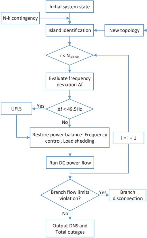
Fig. 1. Algorithm for cascading failure simulations
