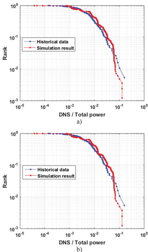
Fig. 6. Cumulative distribution of the DNS obtained with NOMAD with: a) Minkowski distance; b) Kullback-Leibler divergence objective functions.
