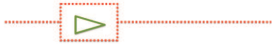
Fig. 5: A simplified visualization of the “moving haven” in an electronic chart. The dotted lines show planned route, and the box show the position where the ship is expected to be according to the plan. The green triangle is the ships AIS symbol based on GNSS input and should be kept in the box. In a 4D electronic chart, a time-slider would allow e.g. a VTS operator with an ability so see all ships’ moving havens, to move forward in time and discover future choke points.
