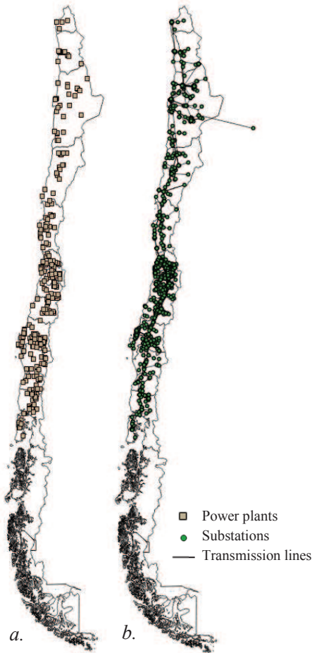
Fig. 1. Map of the Chilean EPN: a) power plants; and b) substations and transmission lines. Notice that the station outside Chile is in Argentina.
